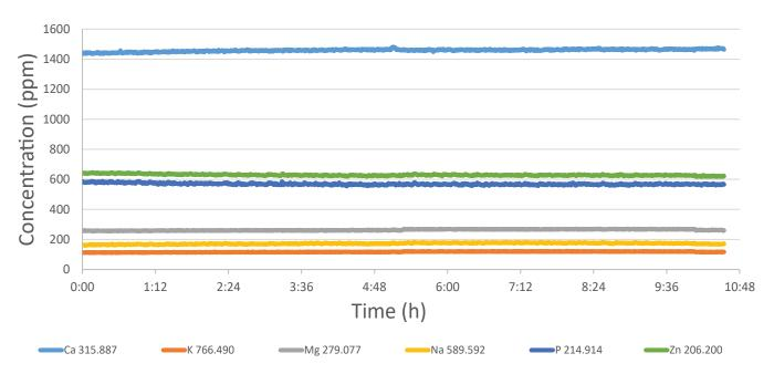
**Figure 5.** SampleSense Oil with 4DXCi autosampler using controlled gas infusion mixing for 23 elements measured over 1764 used motor oil samples in 10 hours and 30 minutes. Stability of six elements with higher concentrations shown above. Lower concentration elements showed similar stability.
