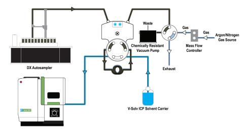
3. Discrete Sample Is Injected into Instrument and ICP Method Is Triggered
