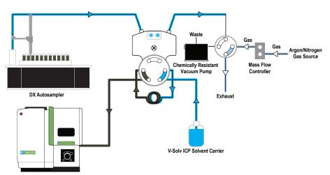
**Figure 1.** SampleSense Oil Controlled Mixing Diagram: (1) Gas infusion valve switches to allow gas flow through SampleSense valve and out the probe. Probe moves into the sample and mixes by gas infusion. (2) With the sample mixed, the gas infusion valve switches and vacuum loading of the loop begins. (3) Once the loop is filled and the sample is sensed, the SampleSense valve switches and sends the sample to the instrument while uptake path is rinsed.
