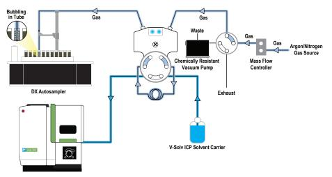
2. Sample Is Rapidly Loaded into SampleSense Valve and Sensed
