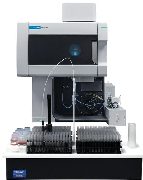
SampleSense Oil Analysis System with Agilent 5900 ICP-OES
