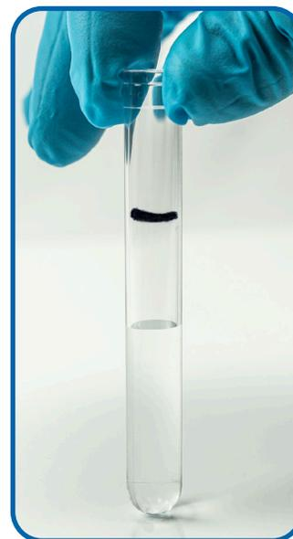
SampleSense Soil consumes < 2 mL of sample. The black line shows the original level of 5 mL extract. Post analysis 3.5 mL remains. Samples can be reanalyzed without re-extraction
