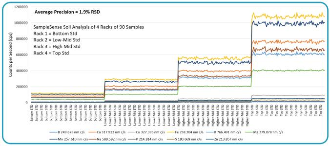
Analysis of 360 samples in 45 minutes. The four levels represent a rack of 90 samples, with each of the four calibration standards levels individually loaded with 5 mL of liquid into each of the 90 positions contained in each rack. Excellent stability observed from within each of the four concentration levels.
