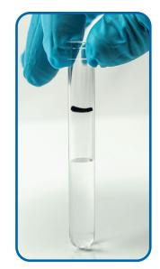
SampleSense Soil consumes < 2 mL of sample. The black line shows the original level of 5 mL extract. Post analysis 3.5 mL remains. Samples can be reanalyzed without re-extraction
