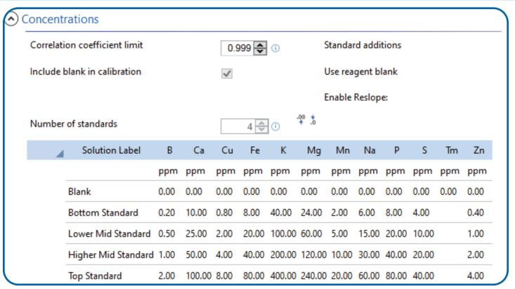
The ICP system was calibrated for the 11 elements of interest with a blank and 4 standards at varying concentrations across the ppm range. The additional element Tm was introduced to assess injection completeness and stability. The linearity of the resulting calibrations are shown on pages 6 and 7.
