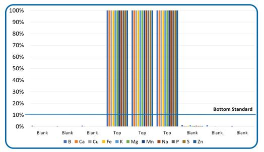
The SampleSense Soil rinse-out immediately reduces all elements to concentrations well below the bottom standard when using the seven and one half second Mehlich-3 ICP procedure. Additional seconds can be added to the rinseout to meet lab requirements. The system can deliver rinse-out factors of 1,000x, 10,000x or more depending on how clear the spray chamber needs to be before the next sample is introduced.
