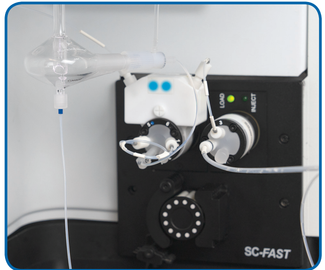
Valve sensors activated, sample is sensed
