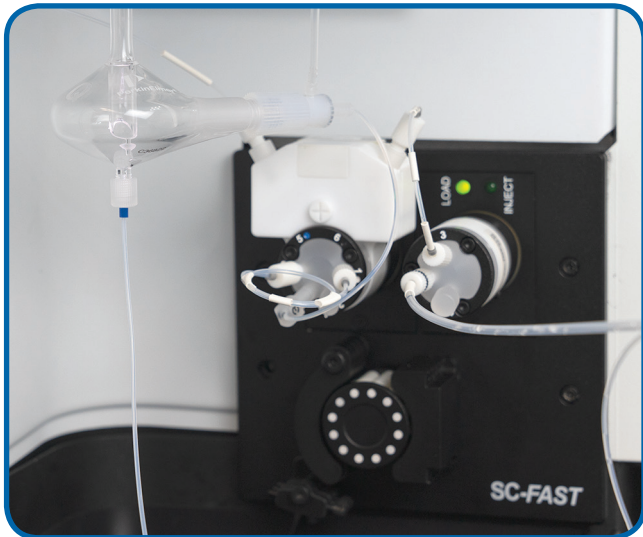
Sample not present, valve sensors not activated
