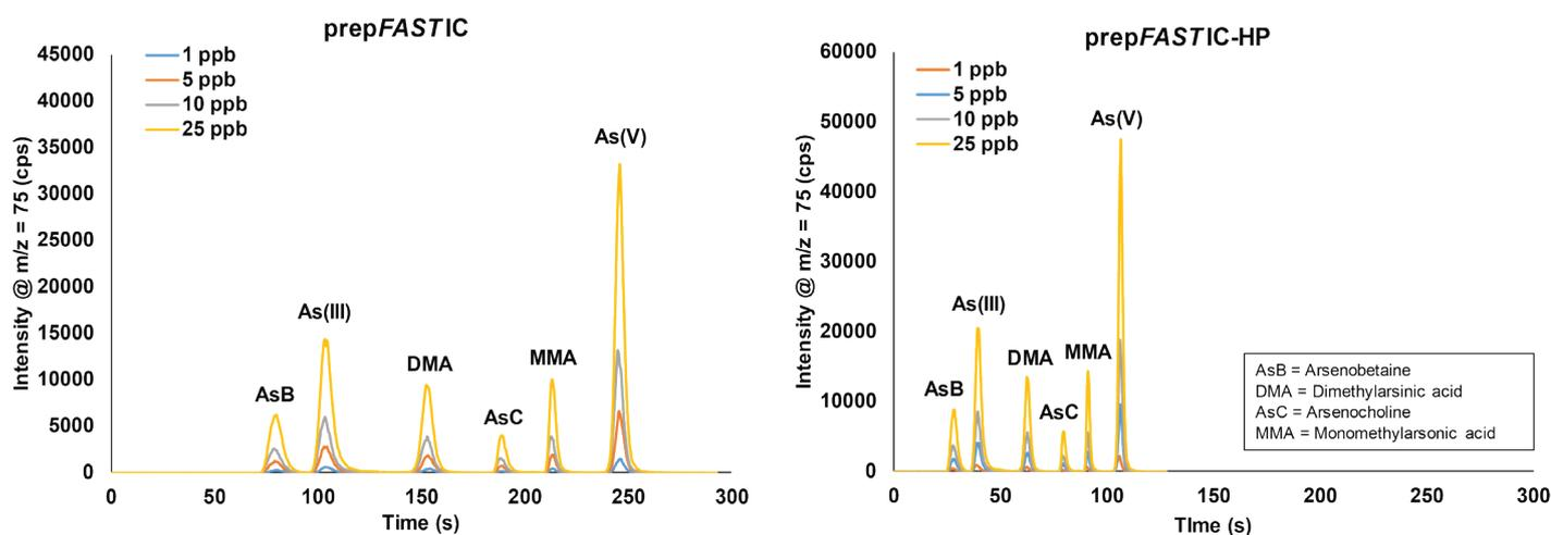
**Figure 1.** Comparison of the arsenic chromatograms obtained from the prepFAST IC and prepFAST IC-HP instruments in combination with an ICP-MS. The prepFAST IC chromatogram was obtained using 0.5 mL/min ammonium carbonate, while the prepFAST IC-HP chromatogram was obtained using 1.5 mL/min ammonium carbonate.
