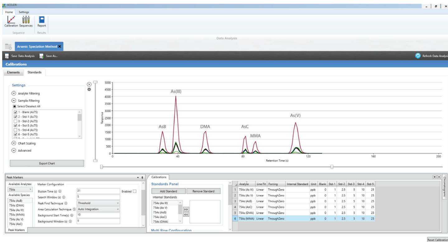
**Figure 2.** Screenshot from Xceleri Software showing the overlay of As species chromatograms. In addition, the automated peak identification and integration parameters are found in the bottom left corner. The calibration curve values for each species are defined in the bottom right corner.
