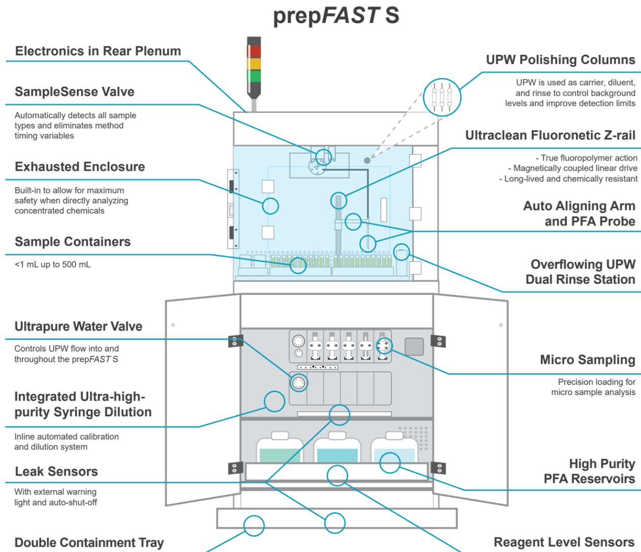
Figure 2. prepFAST S features diagram.
