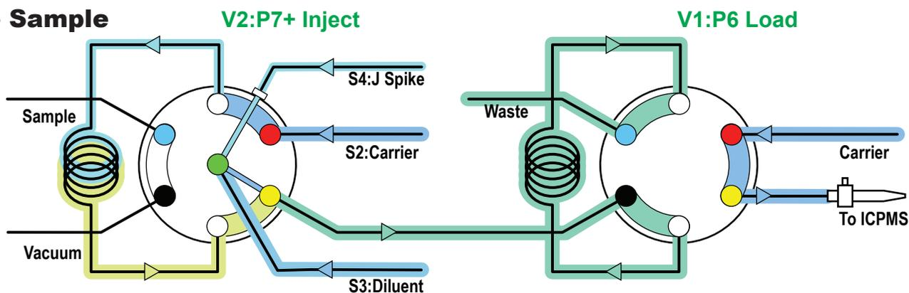
**Figure 2.** The prepFAST system schematic illustrating a two-step process of loading sample into a loop and injecting sample while performing inline dilution.
