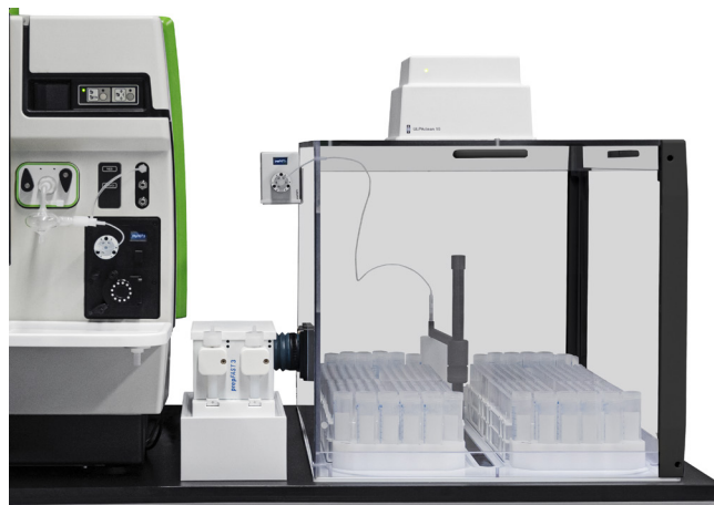
Figure 1. NexION 2000 equipped with a 8DX SampleSense prepFAST 3 autodilution and autocalibration system.
