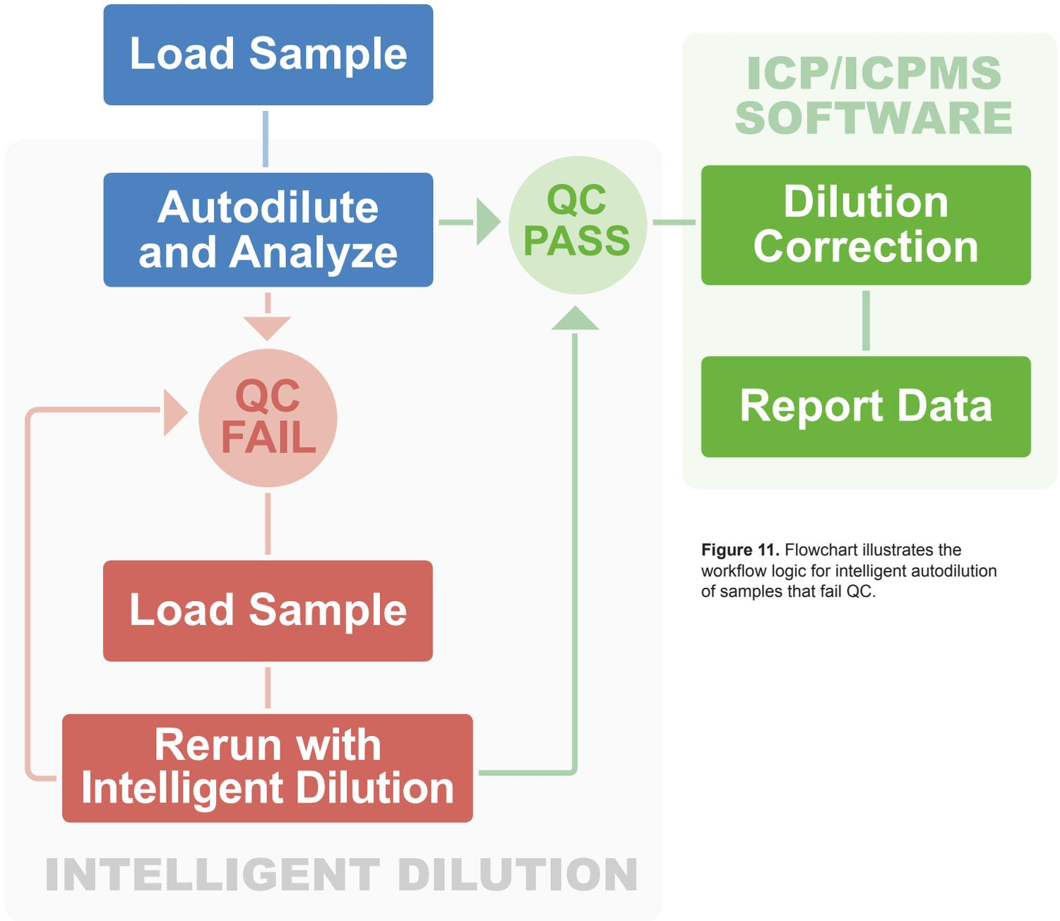
**Figure 11.** Flowchart illustrates the workflow logic for intelligent autodilution of samples that fail QC.
