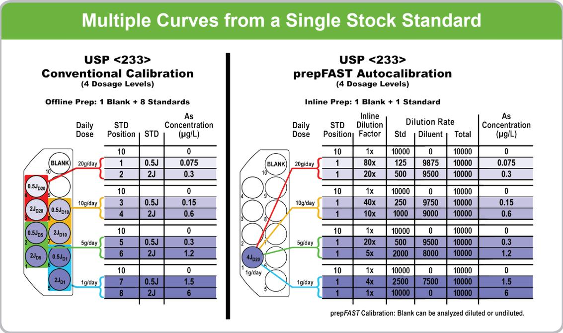
**Figure 5.** USP protocols define a tight calibration range for each drug. In this example multiple drug specific calibration curves are automatically generated from a single stock standard.
