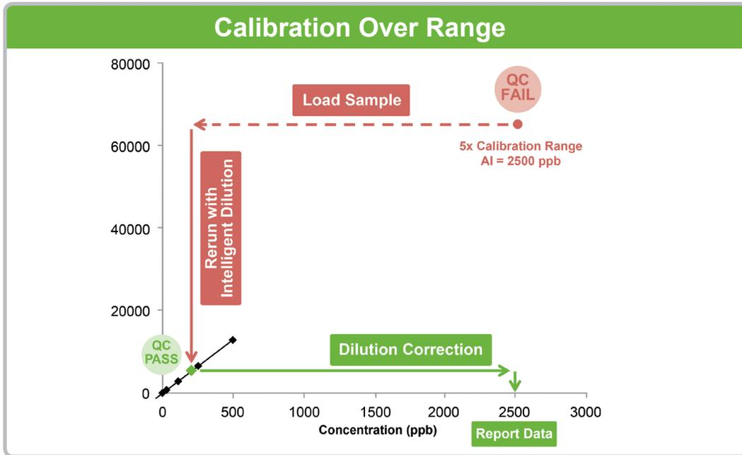
**Figure 12.** prepFAST autodilution in combination with ICPMS QC software can eliminate in-run QC failures. After a QC failure is detected, ICPMS software immediately inserts a new sample line with an intelligent dilution factor. The prepFAST automatically reruns the sample at the new intelligent dilution factor. Advanced prepFAST QC functions are currently available on select instruments.
