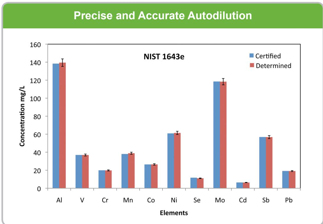
**Figure 10.** Precise and accurate results for concentrations of metals in a Trace Metals in Water Certified Reference Material (CRM, NIST 1643e) are obtained with prepFAST autocalibration and autodilution.
