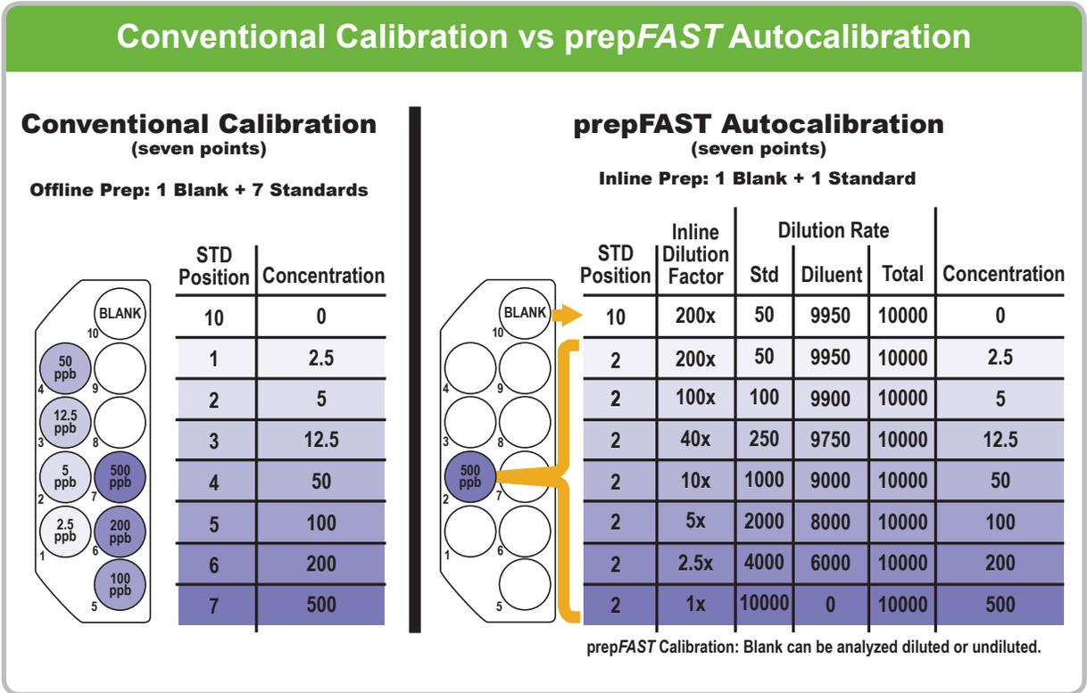
**Figure 3.** Illustration of conventional calibration vs. prepFAST autocalibration function using a single multi-element standard. The full calibration curve is created from vial 2 in the standards rack. Dilution occurs rapidly using small volumes at high flow rates. Sample is then injected at the user's desired flow rate.
