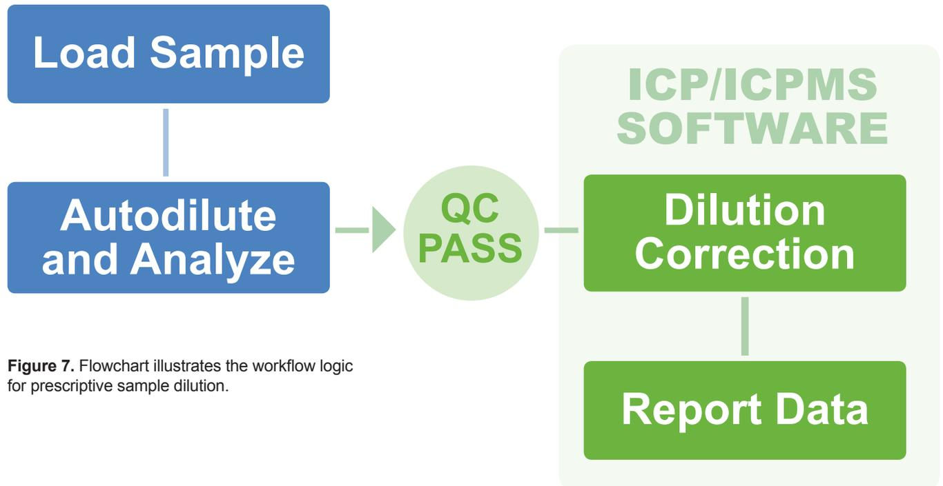
Figure 7. Flowchart illustrates the workflow logic for prescriptive sample dilution.
