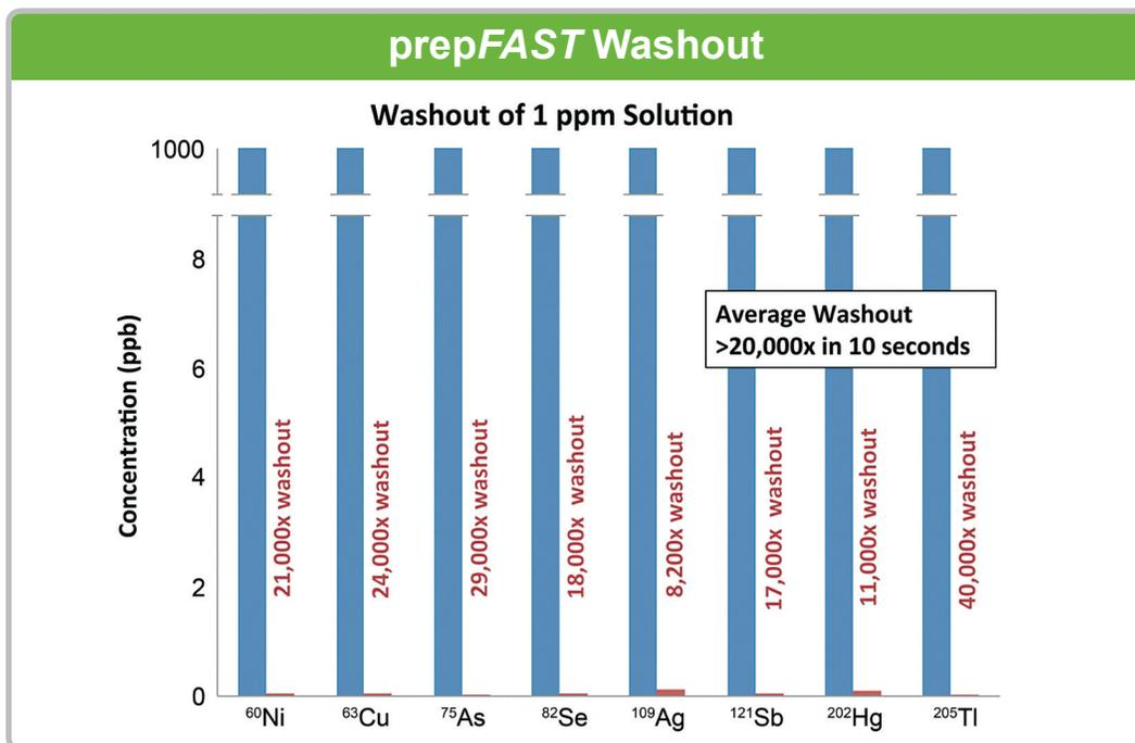
**Figure 13.** For a selection of elements, using the prepFAST, washout greater than 20,000x is achieved in 10 seconds. This is more than sufficient to eliminate any carry-over from the high concentration QC over range sample onto the intelligently diluted re-run.
