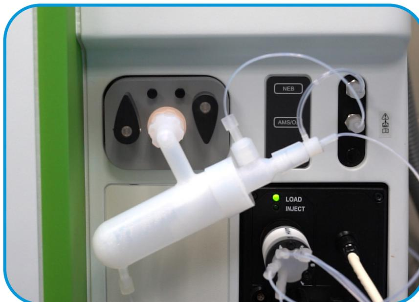
Fluorospray Sample Introduction Kit assembled on NexION 5000 ICPMS
