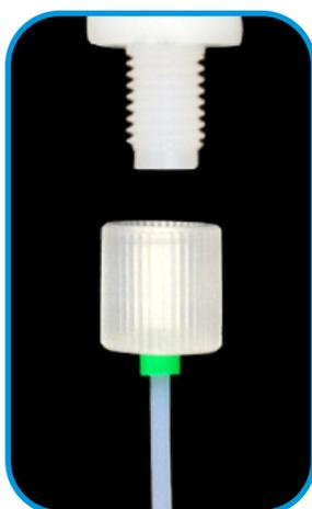
Use one of the sample uptake capillaries or autosampler probes for self-aspiration or directly attach peristaltic pump tubing to the PFA-ST nebulizer
