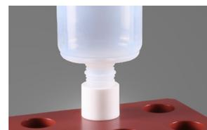
Closeup view of CleanClever in heating well
