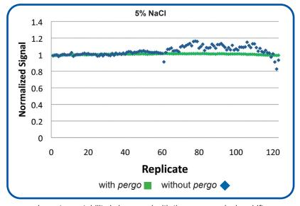
Long-term stability is improved with the *pergo*, reducing drift and extending the length of the analytical run.
