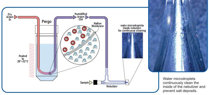
Ar nebulizer gas is humidified using a tube-shaped membrane placed in a PFA water reservoir at atmospheric pressure. The water vapor condenses inside the nebulizer tip, preventing salt build-up.
